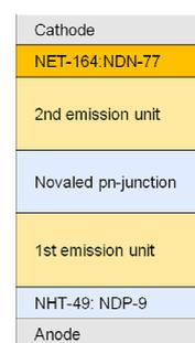
**Fig. 2. Typical tandem white OLED stack architecture with Novaled p-HTL, pn-junction, and the new ETL for low voltage with high efficiency and long lifetime.**
